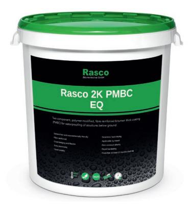
Two component, polymer-modified, fibre-reinforced bitumen thick coating (PMBC) for waterproofing of structures below ground
