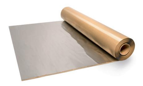
Cold-applied self-adhesive bituminous sealing membrane on aluminium carrier foil for waterproofing of buildings and structures in facade areas, for aeration application, as vapour barrier under screeds in accordance with EN 13970
