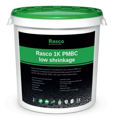
Single component, polymer-modified bitumen thick coating (PMBC) with polystyrene, for waterproofing of structures below ground in accordance with EN 15814 and DIN 18533 - also against water under pressure
