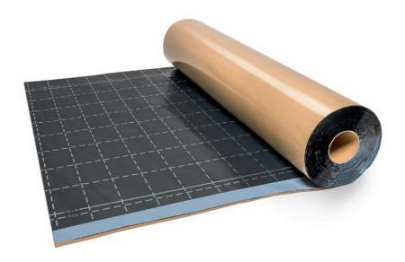
Cold-applied self-adhesive bituminous sealing membrane for waterproofing of structures in accordance with DIN 18533, EN 13969, DIN V 20000-202 and for use as a dampproof course in accordance with EN 14967
