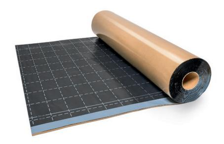
Cold-applied self-adhesive bituminous sealing membrane for waterproofing of structures **especially at high temperatures** in accordance with EN 13967, EN 13969 and EN 14967
